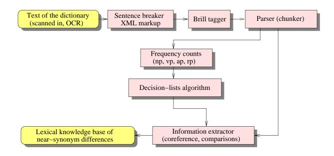
Figure 2.3: The architecture of the extraction module.
