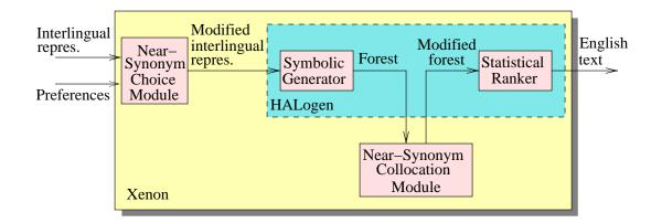
Figure 7.10: The architecture of Xenon extended with the Near-Synonym Collocation module. In this figure the knowledge sources are not shown.
