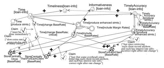
Figure 4: New design with a new requirement.
