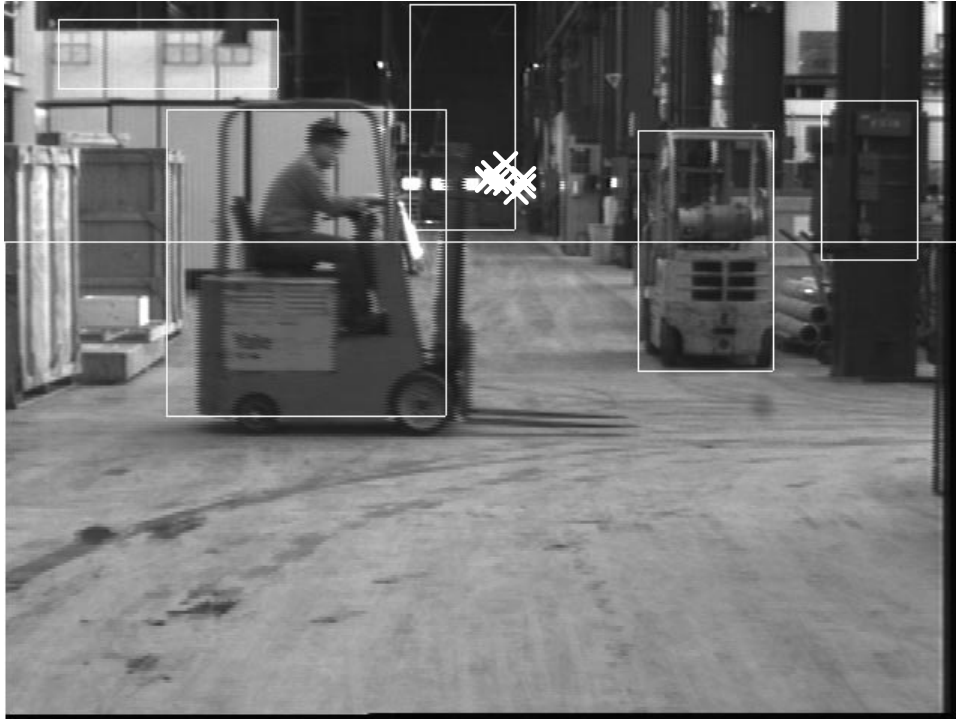
Figure 6. This is a frame from a sequence (of 10 frames) collected by a robot-observer translating roughly along the optical axis in an industrial environment. The forklift and its driver are translating to the right. The boxes indicate image regions for which affine or rational models for optic flow have been fitted. The focus-of-expansion (FOE) of the background motion for each frame in the sequence has been indicated by a 'x'.
