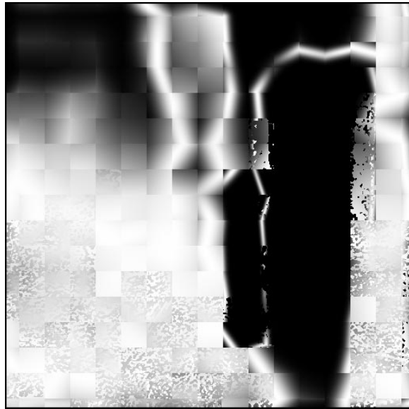
Figure 12. The bottom image shows the probability of each pixel in the dense flow image coming from a region of quadratic flow representing the floor region. The top image is the frame of the original sequence corresponding to the probability map.
