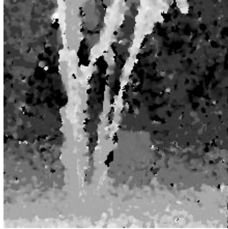
Figure 2.9: SRI tree sequences: Disparity estimates using the local weighted phase-correlated method. The sub-pixel resolution is obtained using linear interpolation of the zero-crossing in the imaginary part of S(x, \tau) .
