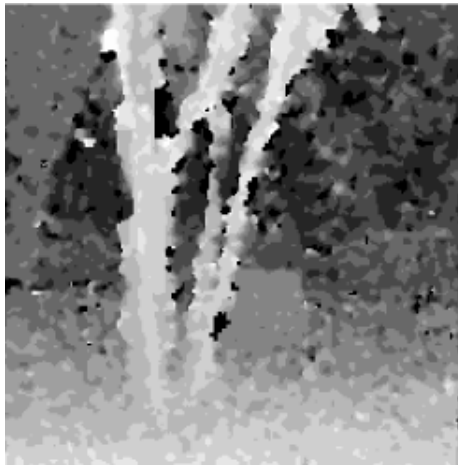
Figure 5.14: Disparity estimate of the SRI tree sequence (frame 2 and frame 4) using the multi-scale Stochastic model. The transition function is a quadratic model. The disparity map has half pixel resolution.
