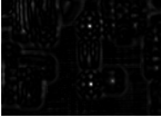
Figure 4. The correlation surface from the top level of the pyramid is shown. Two strong peaks, representing the location of the two instances of the target, are evident. These peaks provide coarse location estimates, which are refined as the algorithm descends through the pyramid.
