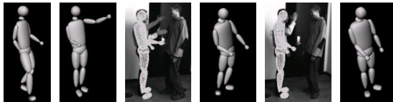
Fig. 7. Exploring system component failure modes. Left (a), (b) shows unfeasible configurations (right hand inside the back and right upper-arm inside the torso) from a run that does not use the flattened embedded priors for physical constraints. Middle (c),(d) and right (e), (f) show two pairs of image projection and 3D configurations when tracking with an embedded model computed without conversation data. The model tracks the beginning of the conversation but eventually loses lock of the arms when the gestures deviate significantly from the training set.
