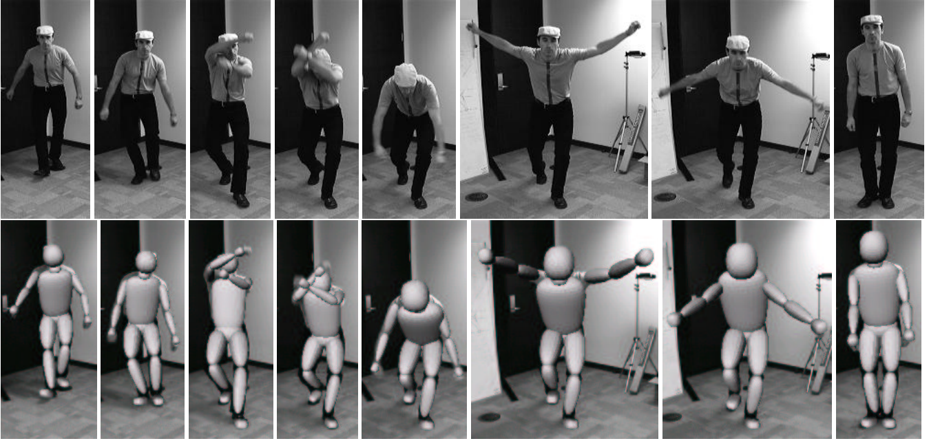
Figure 9: Tracking a 2.5s video sequence containing agile motion in clutter. First row : original Sequence, Second row : one probable model state sequence projected onto image at selected time-steps. See fig. 10 for alternative 3D trajectories.
