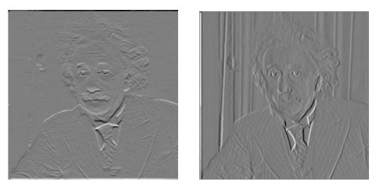
Derivative filters are common in image processing. Here we use crude separable approximations to horizontal and vertical derivatives. They composed of a smoothing filter in one direction (i.e.,  $\frac{1}{4}(1, 2, 1)$ ) and a first-order central difference (i.e.,  $\frac{1}{2}(-1, 0, 1)$ ) in the other.
