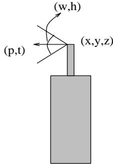
Figure 2: A 2D illustration of the state of the hardware. Where  $(x, y, z)$  is the position of the center of the camera,  $(w, h)$  is the viewing angle size of the camera, and  $(p, t)$  is the viewing direction of the camera.
