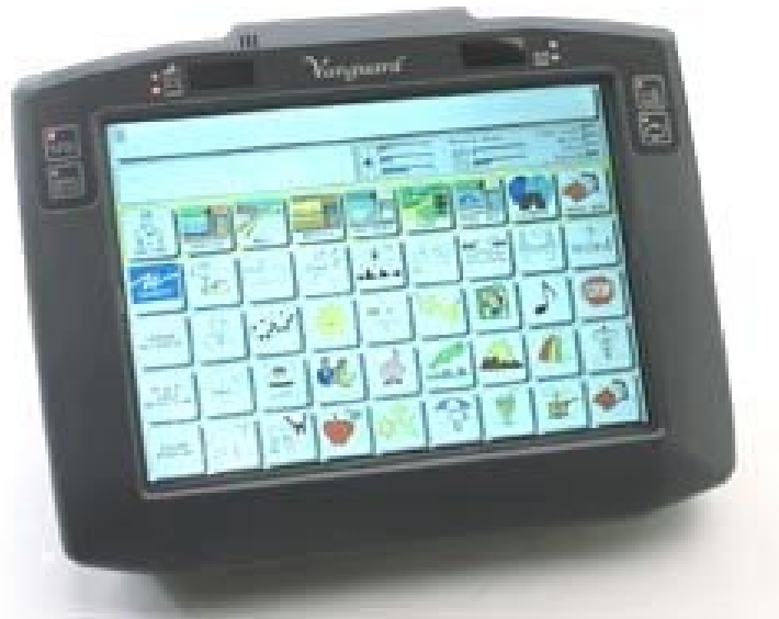
Figure 1.2: Vanguard screen display with its icons for semantic concepts (picture from Aroga Technologies www.aroga.com ).
